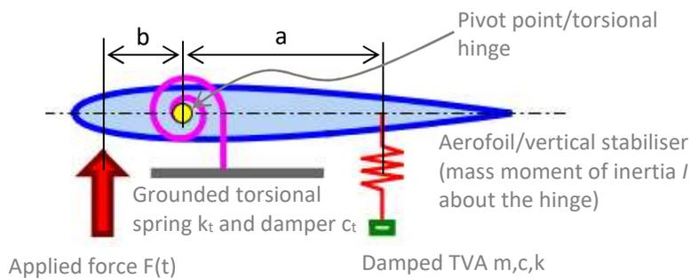
This is a *two degree-of-freedom* problem where the first DOF is realised by the aerofoil pitching and the second DOF is linked with the vertical motion of the TVA mass.
