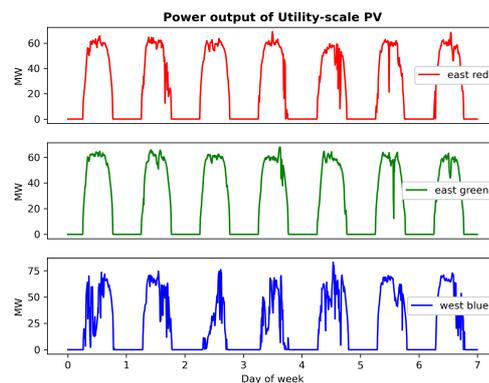
You are given in `solar.csv` some 7-day time-series data for real photovoltaic (PV) power output at 3 different locations in Texas. The three locations are labelled in the file as 'east red', 'east green' and 'west blue' to match the map and plot above.
